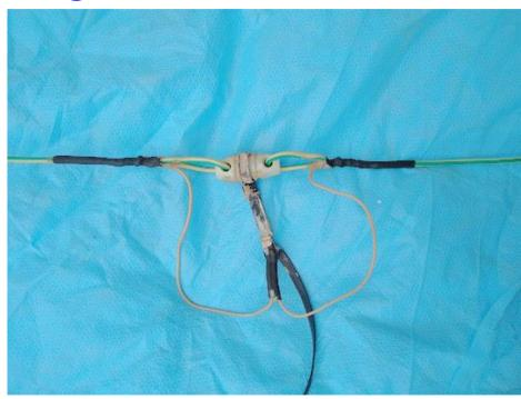
Cable ties and roof and gutter sealant secure a load bearing loop of ribbon. Electric fence insulators can have a groove filed in them tor secure mounting.
