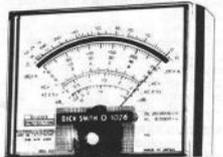
A MULTIMETER CORRECTLY ZEROED FOR MEASURING RESISTANCE
