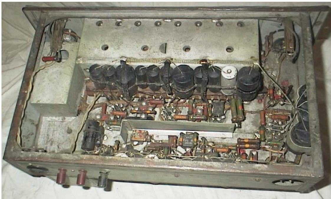
Above: The under chassis view of an AR 7 showing the many old paper capacitors. Photo Ian VK3XI
